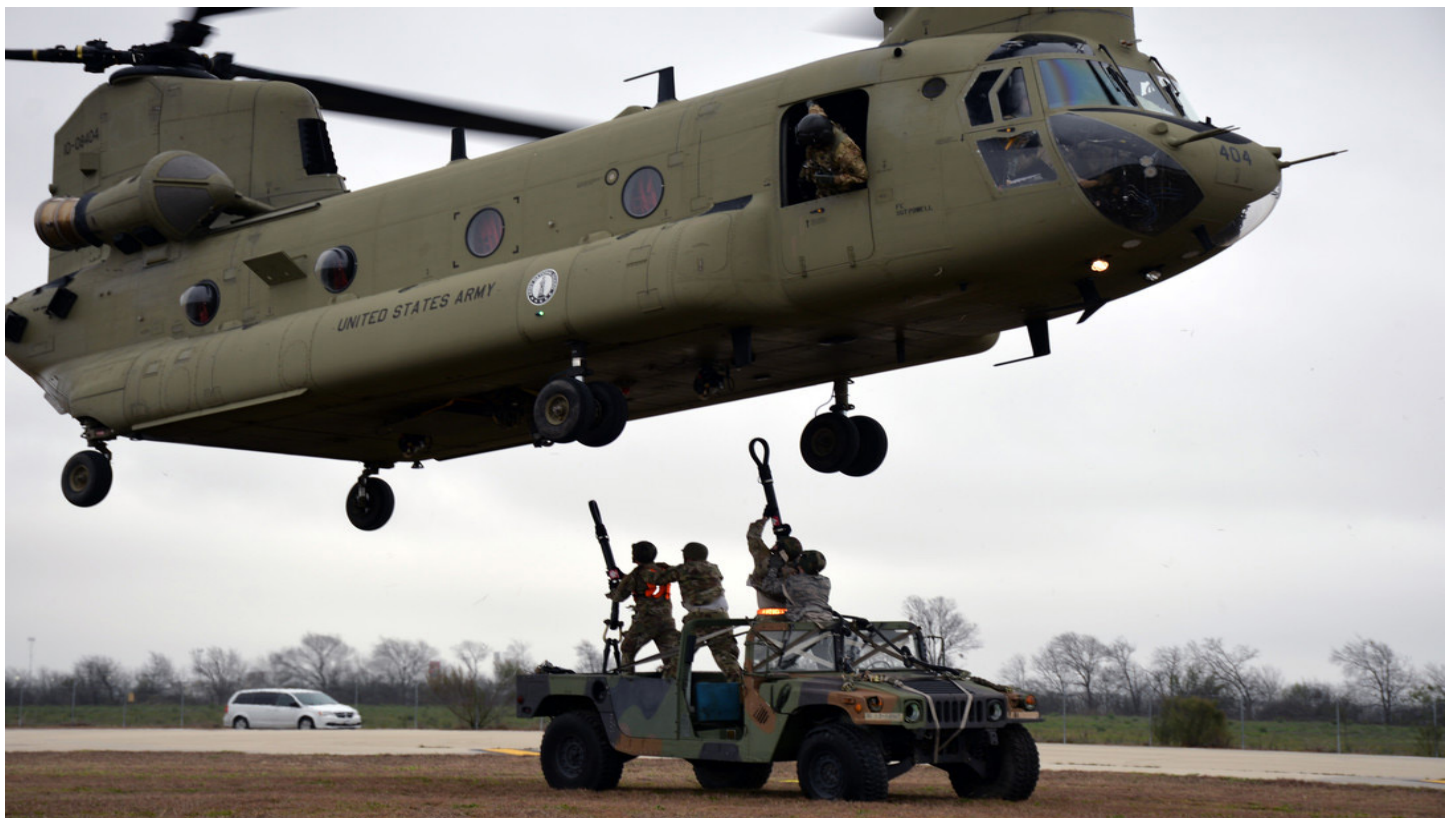
A ground crew prepares to hook a Humvee to a Texas Army National Guard CH-47 Chinook for airlifting during Operation Dust Storm at Martindale Army Air Field, Texas Feb. 1, 2019. The helicopter and ground crews were participating in this joint, total-force training event with active-duty and Reserve Air Force and Army National Guard personnel. (US Air Force photo by MSgt Kristian Carter)
