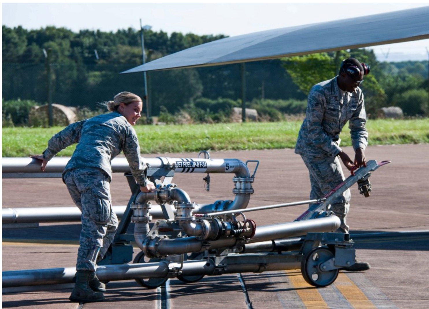
US Air Force SrA Rachel Lockwood and A1C Christopher Broome push a pantograph into place for refueling a B52H Stratofortress after landing at Royal Air Force Fairford, England, 8 September 2016. Lockwood, assigned to the 307th Logistics Readiness Squadron, Barksdale AFB, Louisiana, and Broome, assigned to the 7th Logistics Readiness Squadron, Dyess AFB, Texas, are deployed to RAF Fairford to participate in Exercise Ample Strike, a Czech Republic led, 18 nation live exercise. (US Air Force photo by 1st Lt Monique Roux)
